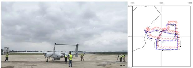
Figure 4 - Left: UAV (model TW328) measurement system developed by Sichuan Tengdun Technology and STI. Right: Flight track and wind observations collected by TW328.
