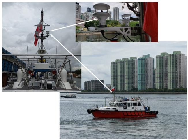
Figure 11 – Dual ultrasonic anemometers were installed on board of a pilot boat travelling over local waters in Hong Kong.
