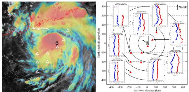
Figure 3 - Wind profiles (radial and tangential components in blue and red respectively) over tropical cyclone Higos collected from the aircraft dropsonde measurement system of HKO (locations of dropsonde marked in triangles) on 18 August 2020 during passage of Typhoon Higos.
