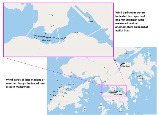
Figure 12 – Display of wind barbs showing (i) one minute mean winds measured by anemometer on board of vessels (longer averaging period is not used as the positions of vessel could be very different over a longer time); and (ii) ten minute mean winds measured by anemometer at land stations or weather buoys at round 16:30 local time on 18 August 2020, when Tropical Storm Higos was about 240 kilometres to the southeast of Hong Kong
