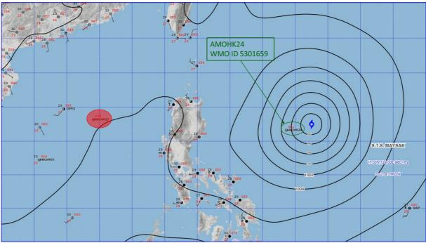
Figure 8 – Maysak (2007) captured by Buoys "AMOHK24" over the western North Pacific at 12 UTC on 29 August 2020. The red-filled ellipse shows the location of another drifter in operation over the South China Sea.
