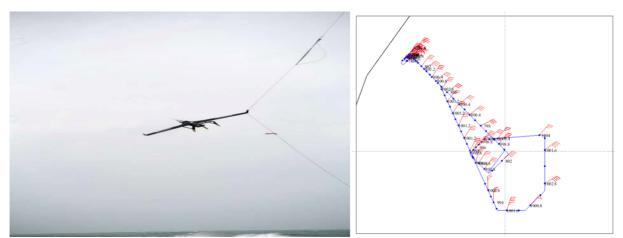
Figure 5 - Left: UAV (model HY30A) measurement system developed by Nanjing University of Aeronautics and Astronautics and STI. Right: Flight track and wind observations collected by HY30A.
